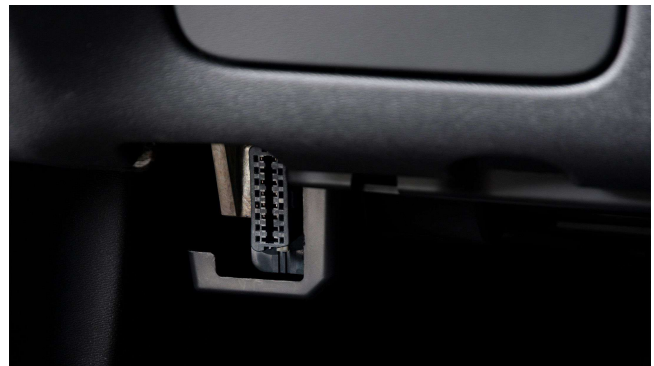
Figure 2: Example of OBD port connector on board a vehicle. It is usually located under the steering wheel, and it has easy access for diagnostic operations.
