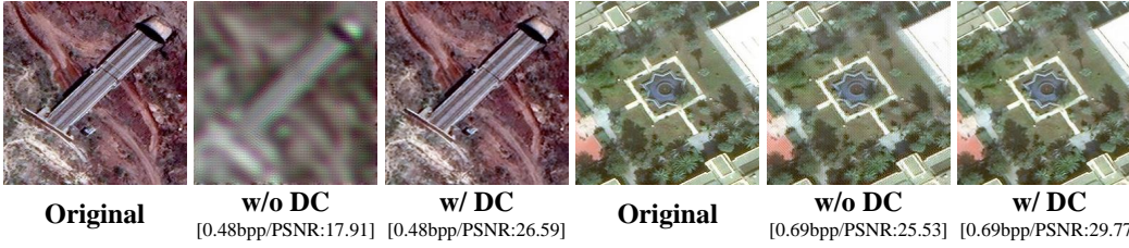
Figure 7: Contrast visual results. “w/ DC” means using of diffusion for compensation during decoding, while “w/o DC” indicates that diffusion compensation was not used during decoding.
