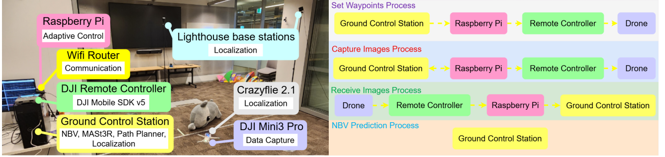
Figure S13. Overview of the real-world drone system. The system uses a drone with an RGB camera for data capture, Lighthouse base stations and Crazyflie for localization, and a Wifi router for wireless communication.
