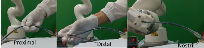
Fig. 5: Intubation methods. From left to right, they are Manual proximal intubation, Manual distal intubation, and robotic intubation.
