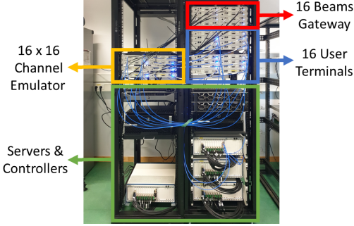
Fig. 7. SDR-based MIMO end-to-end satellite emulator.
