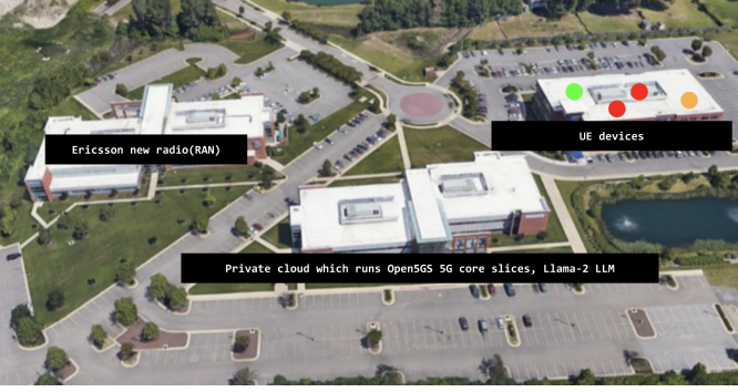
Fig. 3: Proposed large-scale testbed architecture with Ericsson’s new RAN, Open5GS 5G-core, and on-prem Llama-3 LLM in VMASC Virginia US.
