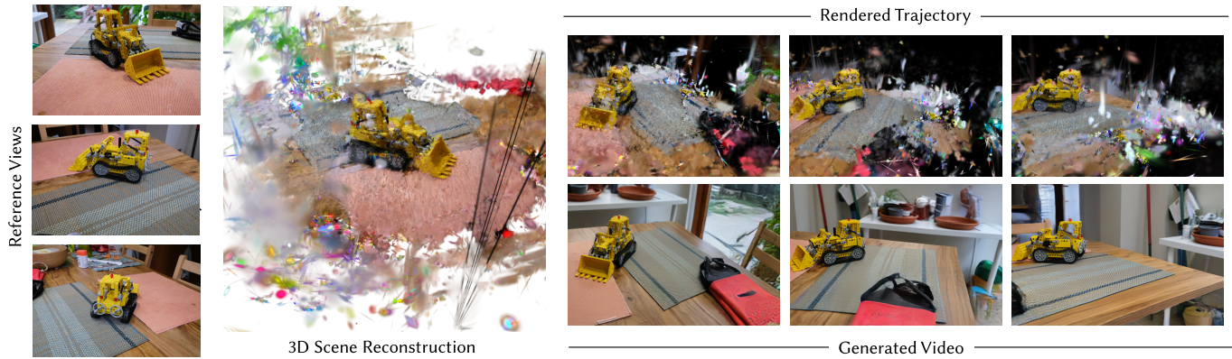
Fig. 1. ARTIFIXER enhances and extends existing 3D reconstructions in a highly efficient and scalable manner. Given an initial reconstruction and optional reference views and text prompt, it auto-regressively generates novel content that maintains a high degree of consistency with existing observations. ARTIFIXER can directly produce hundreds of novel views in a single inference pass or serve as pseudo-supervision to improve the underlying 3D reconstruction. Project page: https://research.nvidia.com/labs/sil/projects/artifixer
