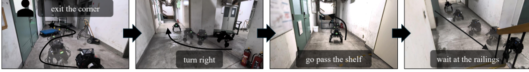
Figure 13: Qualitative snapshots of CoFL-S executing a human-assigned local-instruction sequence in a basement. For each step, we visualize the RGB observation and the assigned local instruction.
