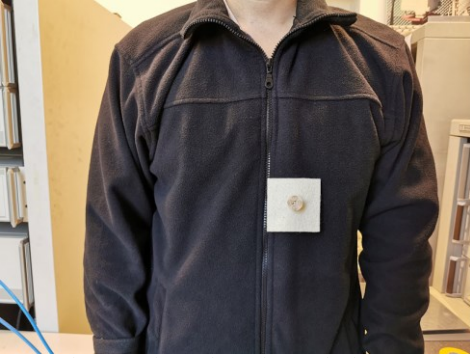
Fig. 13 Measured antenna located on a human body.
