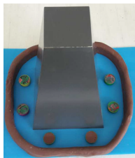
Fig. 5 Wooden mold, encircled by plasticine and plastic coins.
