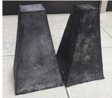
Fig. 4 Developed pyramidal EM absorber made by latex.
