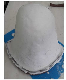
(b) Mask plaster on one side of silicone mold.
