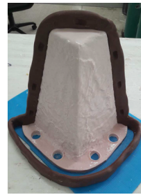
(a) Encircle the silicone mold with plasticine on one side.
