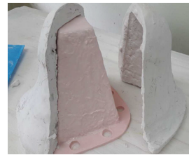
(c) Plaster molds and silicone mold.
