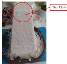
Fig. 6 Mask silicone over the pyramidal wooden mold.
