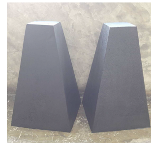
Fig. 8 New proposed absorber obtained from silicone mold.
