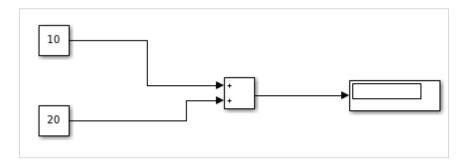
Now click on Run to see the result in the display block. It will add 10 + 20 to give the result as 30 in the display block.
