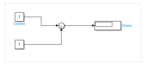
We have created a simple model that has two inputs. These inputs will add up and show the result inside the display.
