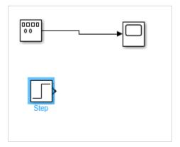
We just have one input for the scope block. Let us increase it to 2 inputs. Right click and open the block parameters.
