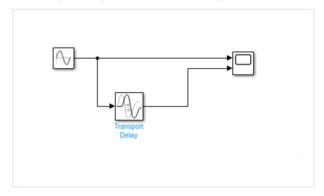
Now run the simulation to see a delay of 3 seconds to the sign wave. Right click scope block and select block parameters to see the display.
