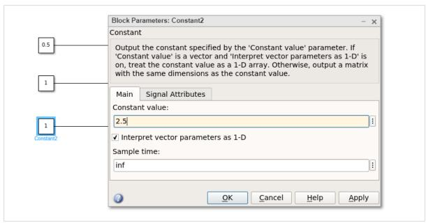
Hence, the first constant value is 0.5, the middle constant value is 1 and the last one is 2.5. The middle constant value 1 will be compared to switch threshold value i.e. 3 as (1 > 3). It will print the value as 2.5 the last constant value.
