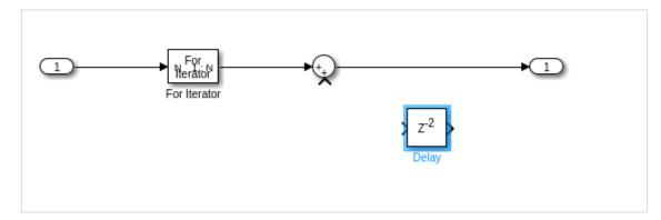
The delay block has to be flipped so that it can be added to the output. We need to give the output back to the sum block so that it can be added with the current iteration.
