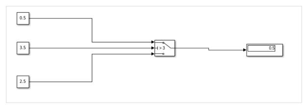
Now, since the value of the middle constant is greater, the value from the first constant is printed in display. If it is less, then the value from the last constant will be printed.
