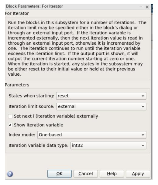
Change the States when starting as reset and Iteration limit source as external. Click on Ok to update the changes.
