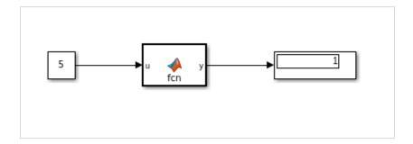
We can see the display as 1, which indicates that the value 5 is an odd number.
