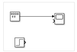
Connect the step input arrow with the scope arrow.
