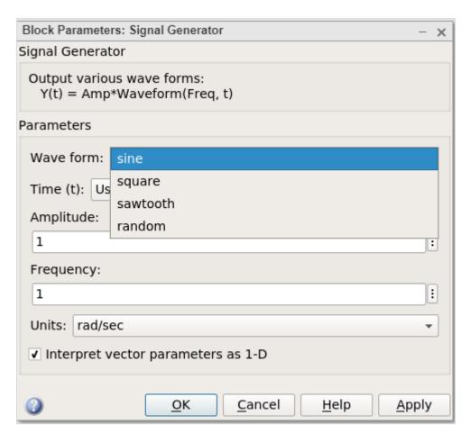
The signal generator can show waveforms like sine, square, sawtooth, random. We will select the square waveform. Let the amplitude and frequency be as 1. Click on OK to update the changes made.
