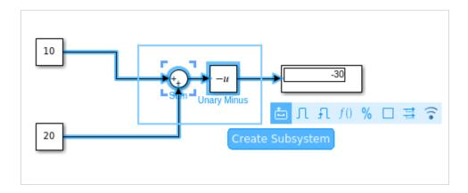
Click on Create Subsystem. Once done, the sum block and the Unary minus block will be converted into a subsystem as shown below:
