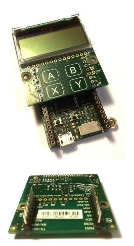
The following video shows how to solder the headers onto the LCD skin. At the end of the video, it shows you how to correctly connect the LCD skin to the pyboard.
