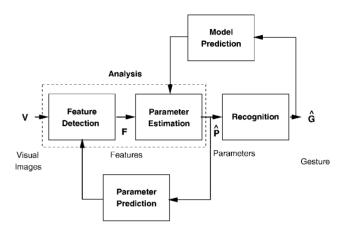
Fig. 8. Analysis and recognition of gestures. In the analysis stage, features *F* are extracted from visual images *V*. Model parameters  $\hat{P}$  are estimated and possibly predicted. Gestures  $\hat{G}$  are recognized in the recognition stage. Recognition may also influence the analysis stage by predicting the gesture model at the next time instance.
