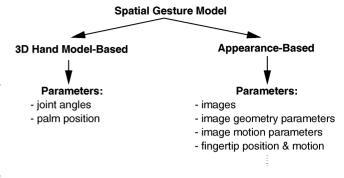
Fig. 5. Spatial models of gestures. 3D hand model-based models of gestures use articulated models of the human hand and arm to estimate the hand and arm movement parameters. Such movements are later recognized as gestures. Appearance-based models directly link the appearance of the hand and arm movements in visual images to specific gestures.
