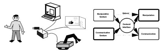
Fig. 9. Applications of gestural interface for HCI. Unlike the gestures in a natural environment, both manipulative and communicative gestures in HCI can be employed to direct manipulations of objects or to convey messages.
