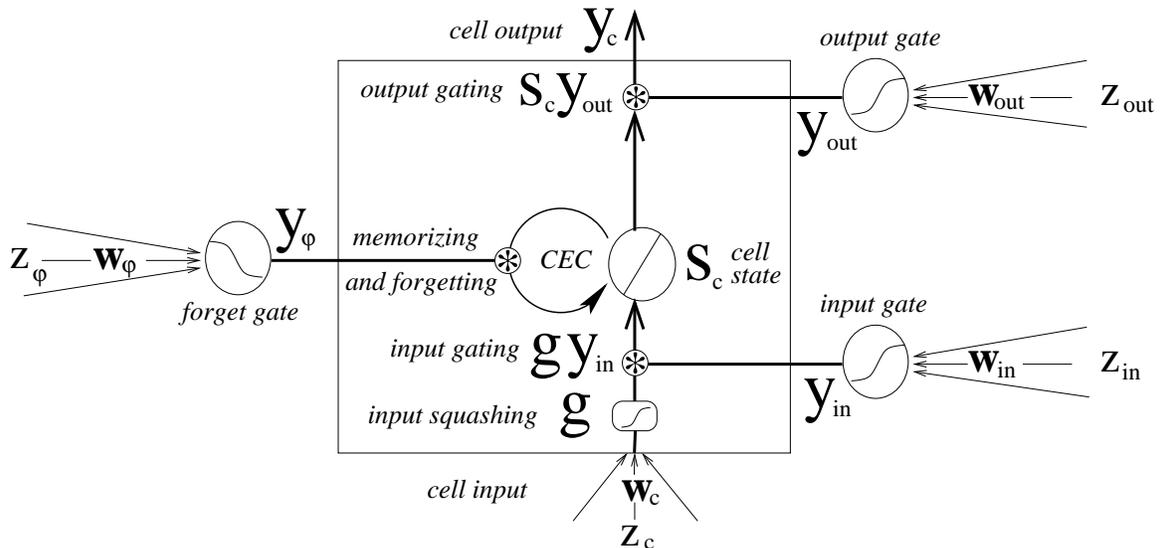
Figure 1: LSTM memory block with one cell (rectangle). The so-called CEC maintains the cell state  $s_c$ , which may be reset by the forget gate. Input and output gate control read and write access to the CEC;  $g$  squashes the cell input. See text for details.
