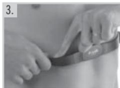
3. Lift the transmitter off your chest and moisten the two grooved electrode areas on the back.
