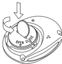
1. Using a coin that sits tight into the back cover groove, open the battery cover by pressing slightly and unscrewing counter clockwise.
