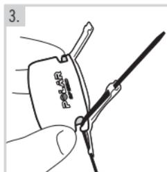
3. Pass the cable ties through the speed sensor and rubber part holes.
