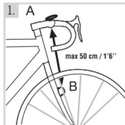
1. Attach the speed sensor to the opposite side of the front fork from the mounted cycling computer. The speed sensor and the cycling computer should be no more than 30-40 cm/ 1'-1'3" apart.
