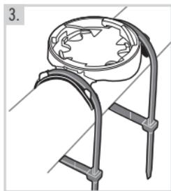
3. Pass the cable ties over the bike mount and adjust them around the handlebar/stem. Secure the bike mount firmly. Cut off any excess cable tie ends.
