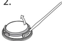
2. Remove the battery cover. The battery is attached to the cover, which should be carefully lifted with a suitable sized small rigid stick or bar, such as a toothpick. A non-metal tool is preferable.
