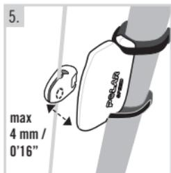
5. Attach the magnet to a spoke at the same level as the sensor. The magnet hole must be facing the speed sensor. Fasten the magnet to the spoke and tighten it loosely with a screwdriver. Do not tighten it fully yet.
