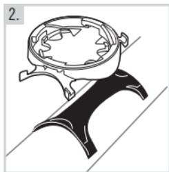
2. Place the rubber part on the handlebar or stem and insert the bike mount on top of it.
