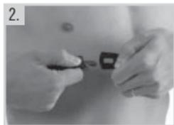
2. Adjust the strap length to fit snugly and comfortably. Secure the strap around your chest, just below the chest muscles, and buckle the strap to the transmitter.
