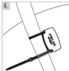
4. Adjust the sensor to the front fork so that the POLAR logo faces outwards. Adjust the ties loosely. **Do not tighten them fully yet.**
