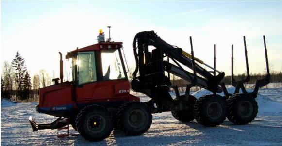
Figure 1: Forest machine with articulated steering
