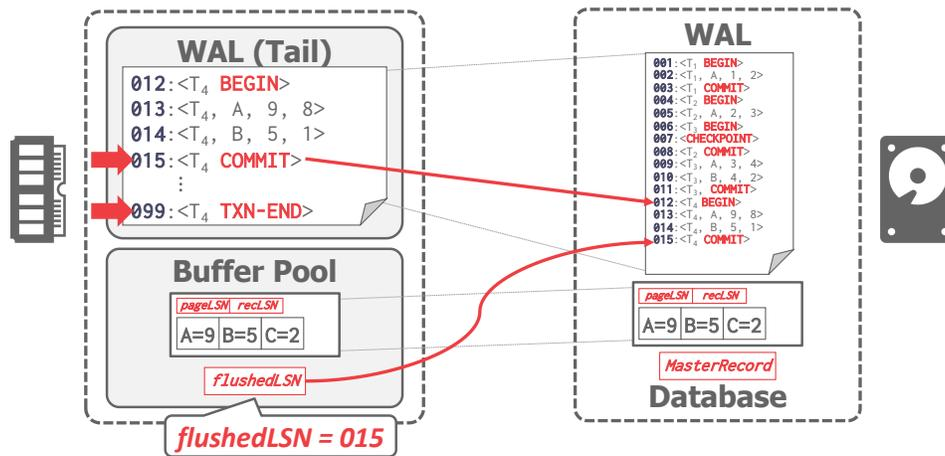
**Figure 2: Transaction Commit** – After the transaction commits (015), the log is flushed out and the flushedLSN is modified to point to the last log record generated. At some later point, a transaction end message is written to signify in the log that this transaction will not appear again. Then we can trim the in-memory log up to flushedLSN.
