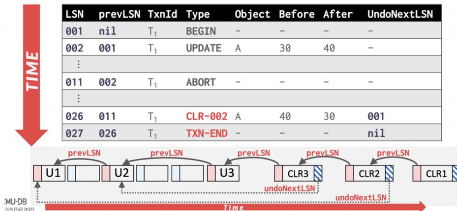
**Figure 3: Transaction Abort** – The DBMS maintains an LSN and prevLSN for each log record that the transaction creates. When the transaction aborts, all of the previous changes are reversed. After the log entries of the reversed changes make it to disk, the DBMS appends the TXN-END record to the log for the aborted transaction.
