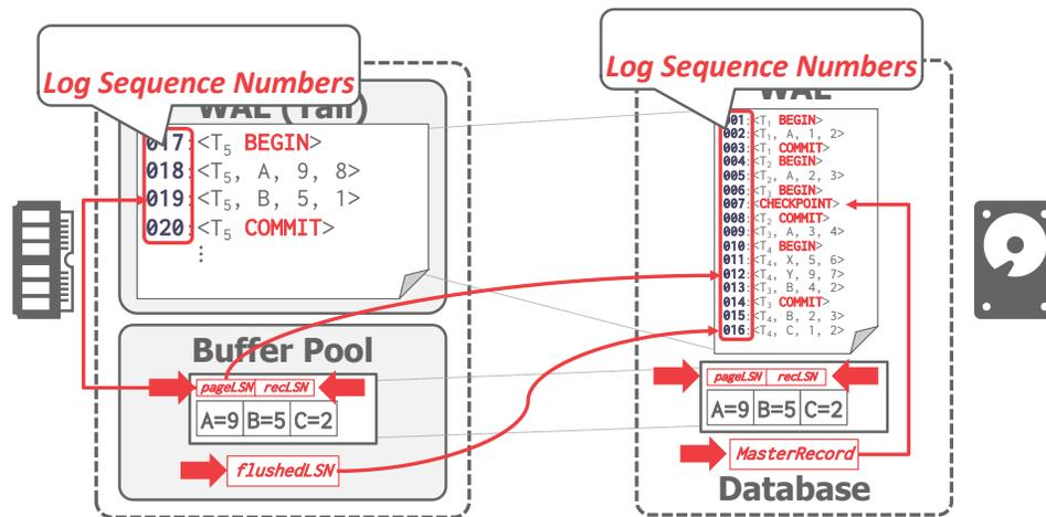
**Figure 1: Writing Log Records** – Each WAL has a counter of LSNs that is incremented at every step. The page also keeps a pageLSN and a recLSN, which stores the first log record that made the page dirty. The flushedLSN is a pointer to the last LSN that was written out to disk. Before the DBMS can write page  $i$  to disk, it must flush log at least to the point where  $pageLSN_i \leq flushedLSN$ . The MasterRecord points to the last successful checkpoint passed.
