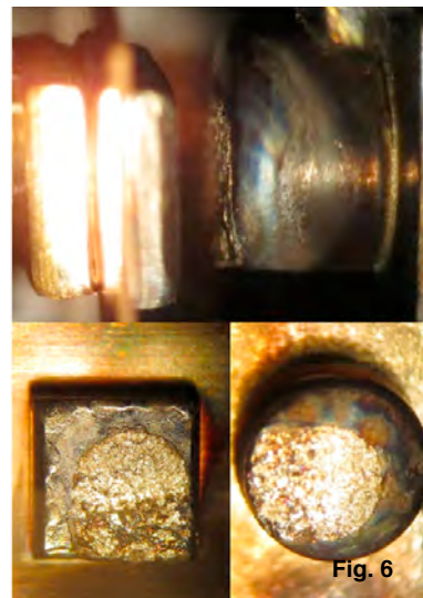
Fig. 6 shows side and face views of contacts from a relay operated with a NOsparc arc suppressor across the contacts. This relay completed 100,000 cycles.
