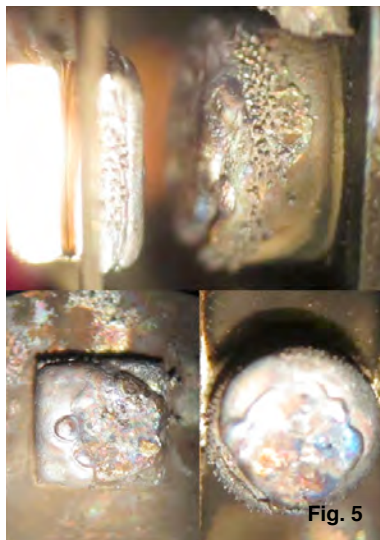
Fig. 5 shows side and face views of contacts from a relay operated with a typical RC snubber across the contacts. This relay completed 100,000 cycles.
