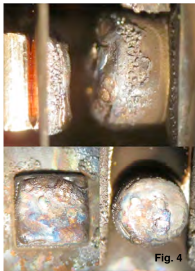
Fig. 4 shows side and face views of contacts from a relay operated without any arc suppression element. This relay completed 88,265 cycles.
