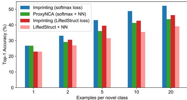
Figure 6. Top-1 accuracy of 100-way classification on novel classes of CUB-200-2011. Imprinting averaged embeddings with a softmax loss (blue bars) outperforms storing all individual embeddings with a nearest-neighbor classifier (green). By comparison, embeddings trained with the lifted structured loss do not perform as well as with the softmax loss (red and pink).
