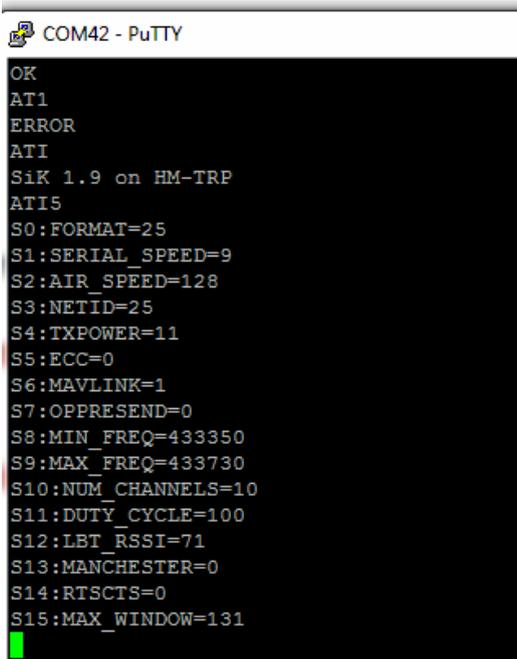
**Figure 33: Send AT commands to Radio Modem**
