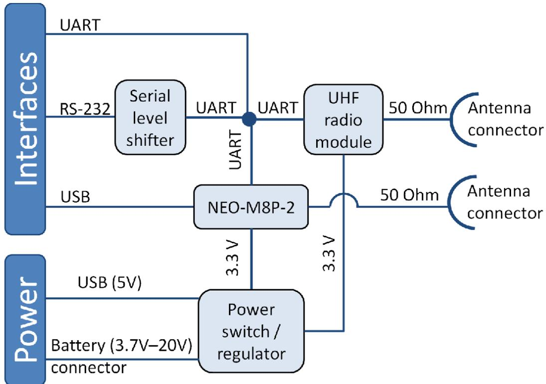
Figure 27: Block diagram of the C94-M8P application board
