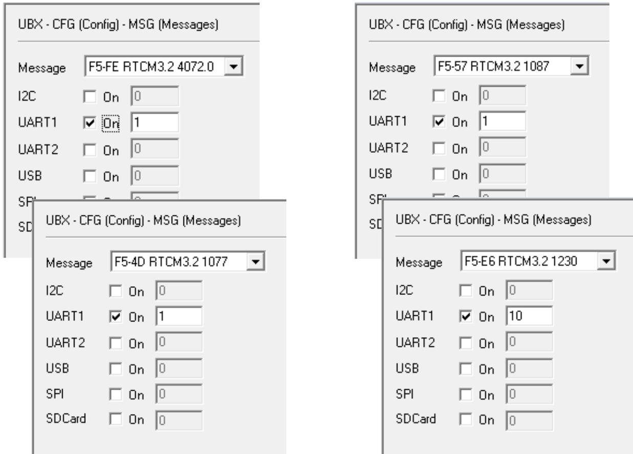
Figure 10: For a GPS+GLONASS setup, enable the RTCM messages 4072, 1077, 1087 and 1230 on UART1 port
