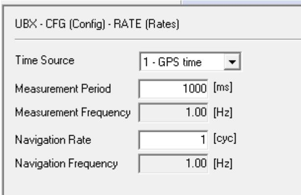
Figure 13: Navigation rate set to 1 Hz
