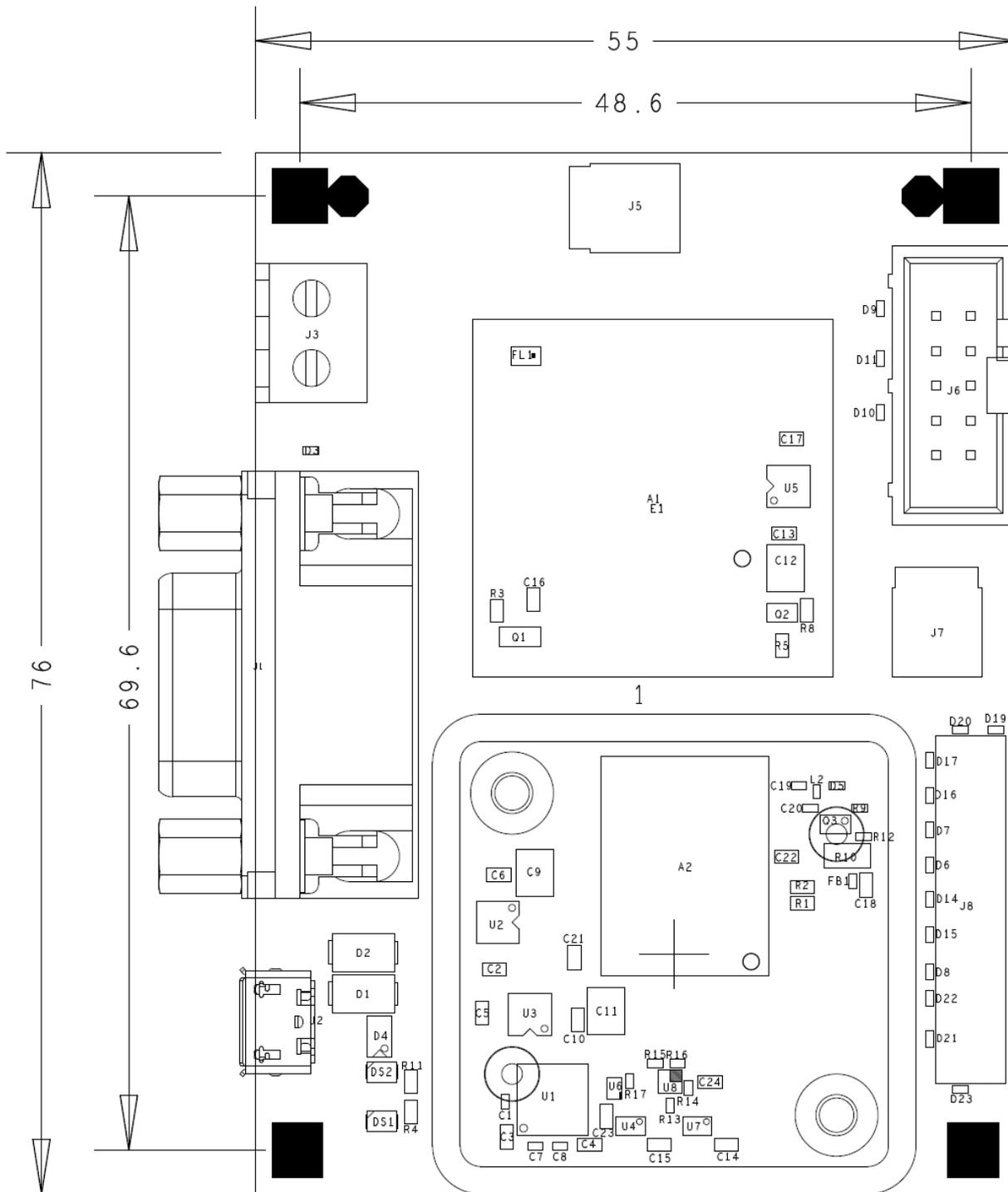
Figure 28: Board Layout of C94-M8P-D/E Application Board
