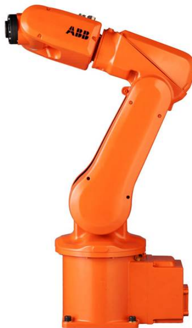
Figure 1: The ABB IRB 120 industrial 6-DoF Manipulator
